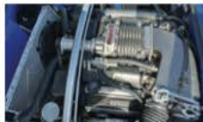
Sprintex supercharger is of the Roots type, with this addition increasing the V8's power by almost 100kW.
