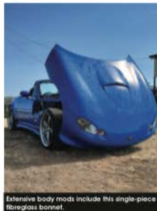
Extensive body mods include this single-piece fibreglass bonnet.
