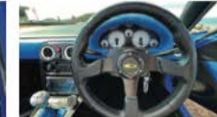
Gauge faces were changed to Bullet-branded items that included a 300km/h speedometer.
