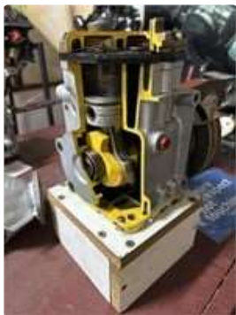
526 Cut Down Air Conditioner Pump
