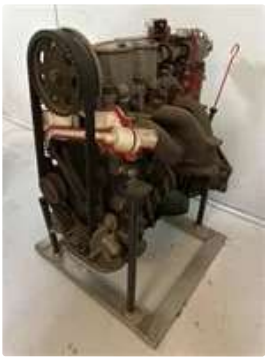
313 Engine Cut Down Holden Camira on Stand
