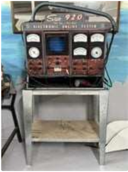
309 Early Electronic Engine Tester SUN 920 On Stand
