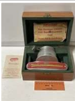
645 Vintage Replex REPCO King Pin Inclination Gauge
