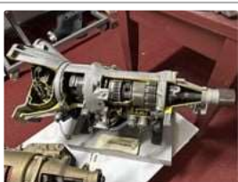
529 Cut Down Holden VL Commodore Gear Box
