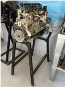
308 Engine Cut Down Holden Grey Motor on Stand
