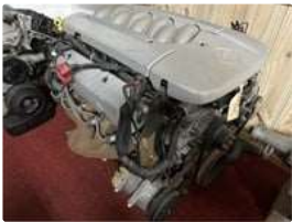
518 5 Ltr Holden V8 Engine Complete w/- Auto Transmission
